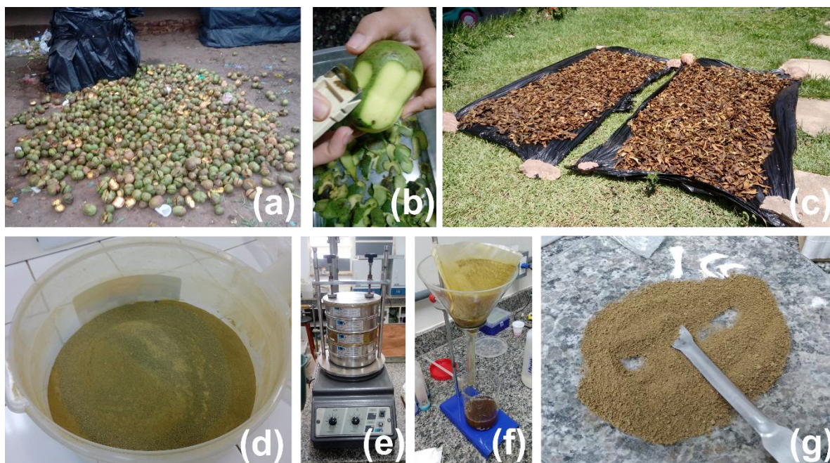
Figure 1: CCB adsorbent preparation steps. (a) Collection and washing of CCB waste. (b) Peeling. (c) Natural drying. (d) Crushing. (e) Granulometric adjustment (32mesh). (f) Washing the crushed material. (g) Oven drying and stock for use in analysis.
